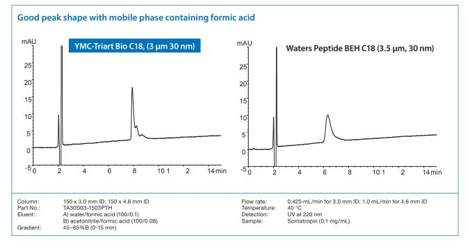
YMC-Triart Bio C18 is suitable for highly sensitive analysis and structural analysis of proteins using LC/MS since good peak shapes in mobile phase containing formic acid can be achieved.
