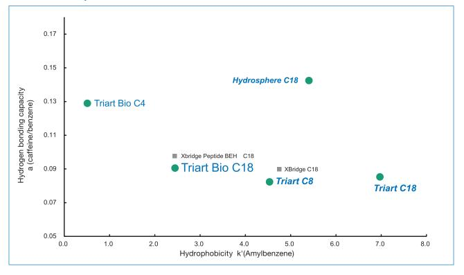
YMC-Triart Bio C18 shows a selectivity between that of YMC-Triart Bio C4 and regular YMC-TriartC18/C8 with 12 nm pore. This feature perfectly supplements the existing products.
